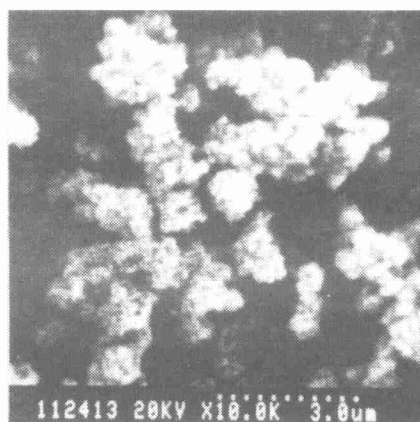
Fig.4 Morphology of La-Co alloy film obtained at 3 \text{ mA/cm}^2 observed by SEM
