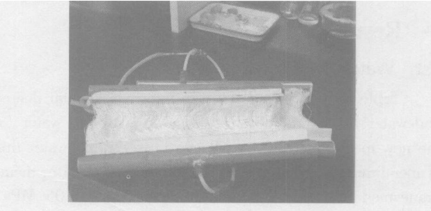
Fig 2 Fiber hollow membrane module
