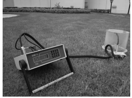
图 1 冠层同化箱和 CO 2 气体分析仪 Fig. 1 Image of canopy assimilation chamber and environmental gas analyzer for CO 2
