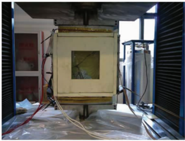
图 5 绝热结构损伤检测温度-载荷联合试验布置图 Fig. 5 Layout of temperature-load combined test for damage detection of insulation structure
